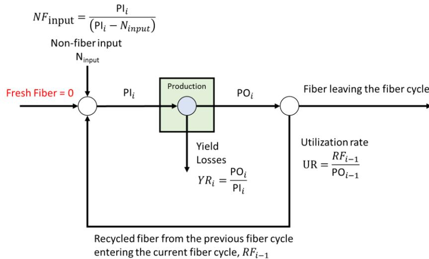
Figure 1. Fiber cycle mass balance for cycle  $i$
